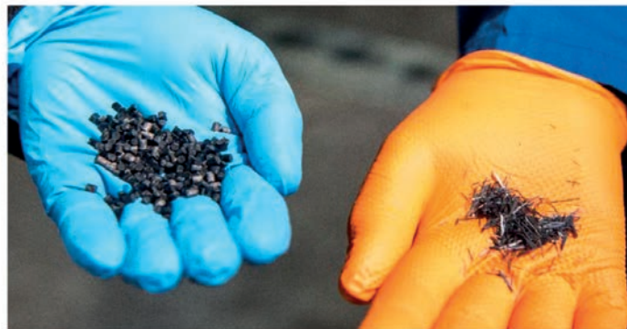
Fig. 3. Recycled/pyrolyzed carbon fiber by Global EnerTec AG (right) and new thermoplastic compound containing recycled carbon fibers (left)
