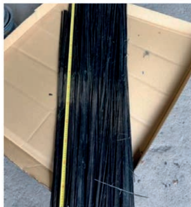
Fig. 11. Carbon fibers obtained in pyrolysis process which were cut out of the central strap in wind turbine blade
