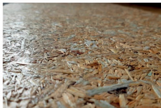
Fig. 10. Chipboard panels made from recycled end-of-life composites
