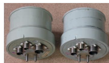
Fig. 2. Protection and execution mechanism before disassembly (WITU)
