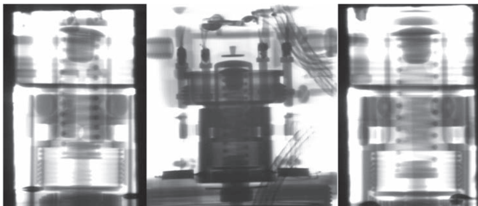
Fig. 10. X-ray of the WDM-5 type combat booster (WITU)
