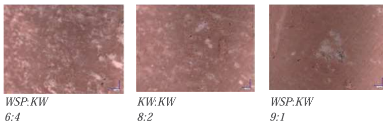
Fig. 7. The surface of briquettes made of high calcium filter sludge mix with limestone (Photo: B. Kosturkiewicz)
