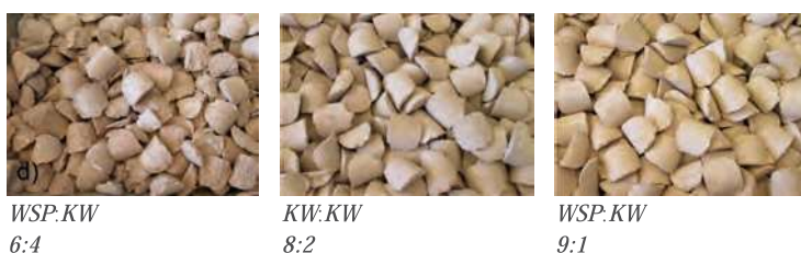
Fig. 4. Photos of briquettes obtained from mixtures of high-calcium filter sludge and limestone (Photo: B. Kosturkiewicz)
