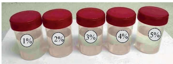
Fig. 4. Images of wastewater samples from the poultry industry treated with variable doses of natural zeolite from Turkey (doses of 1–5% by mass)
