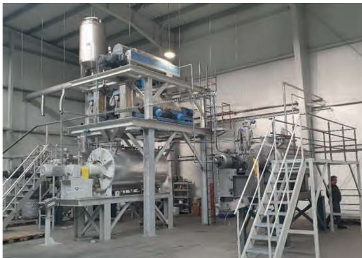
Fig. 3. Photo of the pilot plant constructed on the premises of Altempo with a processing capacity of over 300 kg/h of LDPE-Al laminate
