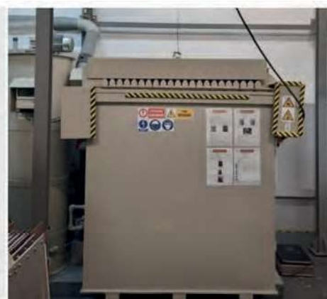
Fig. 1. An industrial research stand for testing the electrowinning of metals from the solution after acid reductive leaching of battery mass from lithium-ion cells
