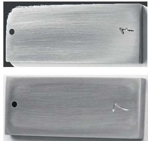
Fig. 1. Original appearance of the ground and polished sample taken from the X65C pipe: 1 (without weld) and 7 (with weld)
