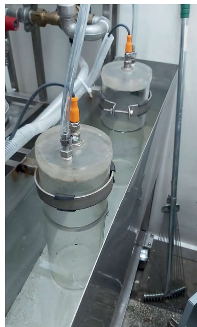
Fig. 3. Biogas collecting vessels with gas throughput sensors
