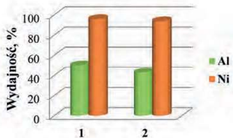
Fig. 6. Efficiency of nickel and aluminum sorption process from solutions after mineralization of 1 – fresh, 2 – used catalysts, at pH 5.0
