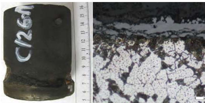
Fig. 3. Fragment of a boiler tube: a) thinning, b) microstructure of the wall on the outer side
