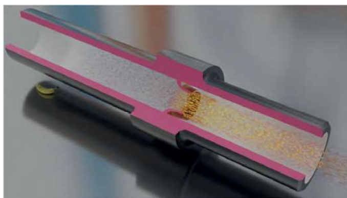
Fig. 1. Visualisation of the cross-section of the ISA 1932 measuring nozzle and the velocity vectors obtained during simulation
