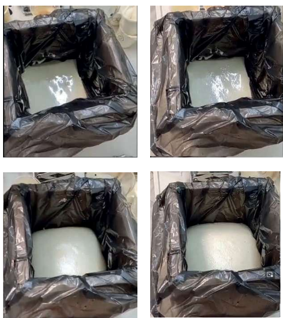
Fig. 6. Foaming of PUR foams using recycled polyol from PUR depolymerization Rys. 6. Spienianie pianek PUR z wykorzystaniem depolimeryzatu PUR
