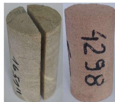
Fig. 1. An example of rock samples used for studies: limestone from A deposit (on the left), sandstone from B deposit (on the right)
