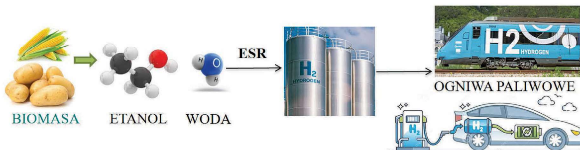
Fig. 1. Schematic diagram of the production and use of hydrogen from the ESR process
