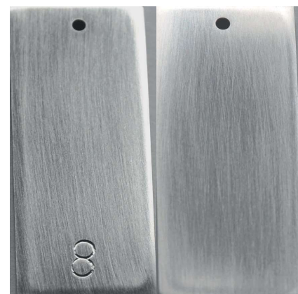
Fig. 3. Front and back surface of specimen 8 of N80 steel, before test 2
