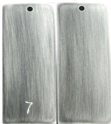
Fig. 2. Front and back surface of specimen 7 of N80 steel, before test 1
