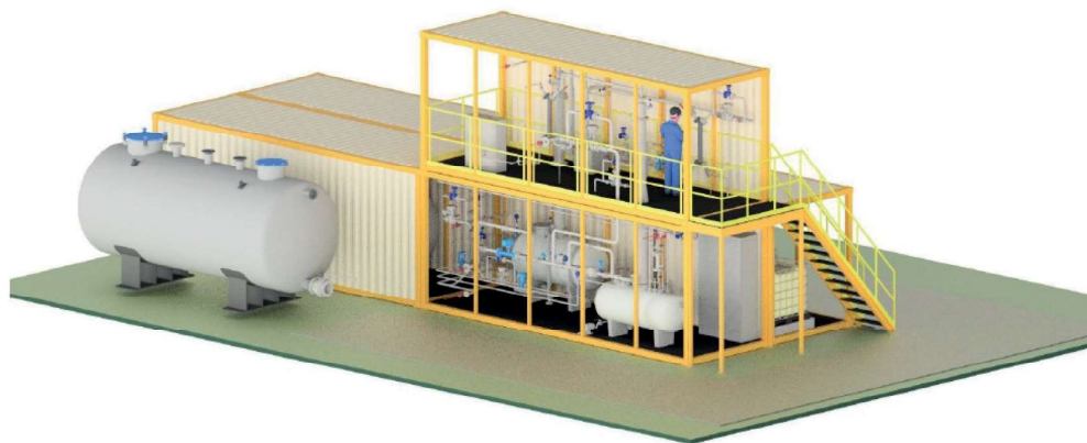
Fig. 4. Modular installation for separation of clean green carbon dioxide from biogas and exhaust gases
