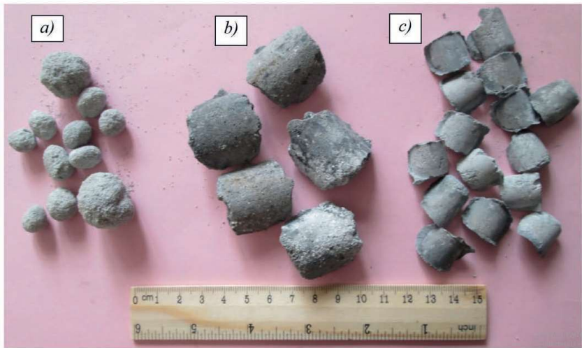
Fig. 1. Granules and briquettes obtained from compaction devices: a) disc granulator, b) roller press LPW 450, c) roller press LPW 250 (Photo: Bogdan Kosturkiewicz)
