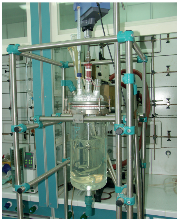
Photo 3. Set of apparatus for the production of didecyldimethylammonium lactates on a large laboratory scale (Photo: Ł-ICHP)
