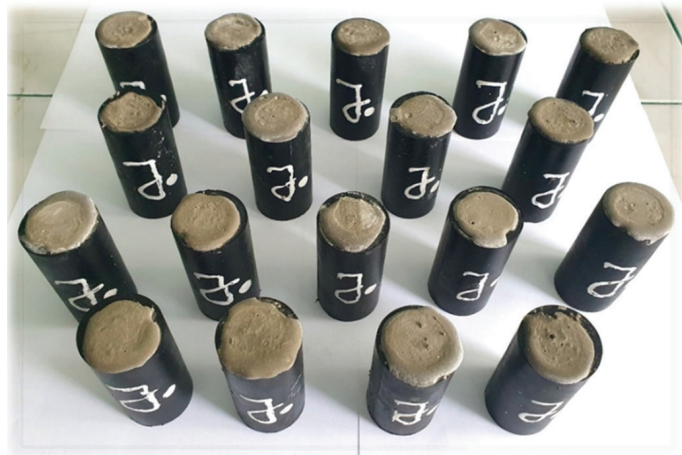
Fig. 1. Samples of hardened cement slurry prepared for testing
