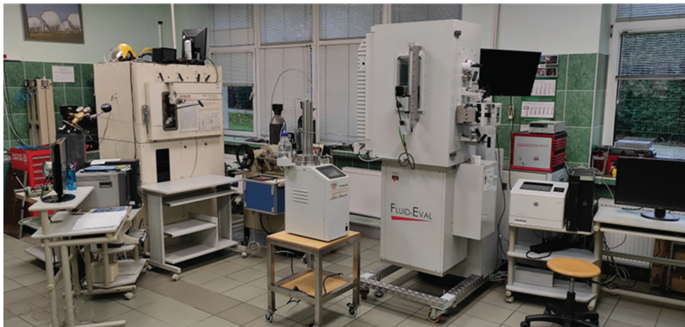
Fig. 2. Integrated fluid and rock testing equipment for reservoir PT conditions, Chandler Eng. PVT System and VINCI Fluid Eval
