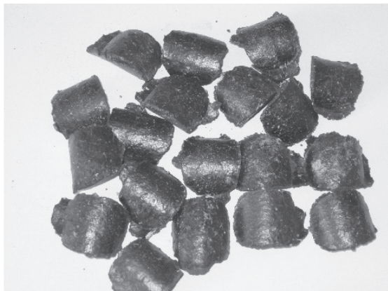
Fig. 3. Briquettes obtained from a mixture of waste basalt (brown coal, waste basalt, coffee grounds and municipal sewage sludge)
