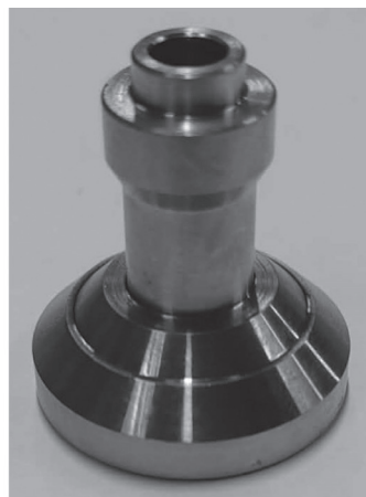
Fig. 1. Appearance of the parts used in the processes: a) made of 16MnCr5 steel, b) made of 42CrMo4 steel
